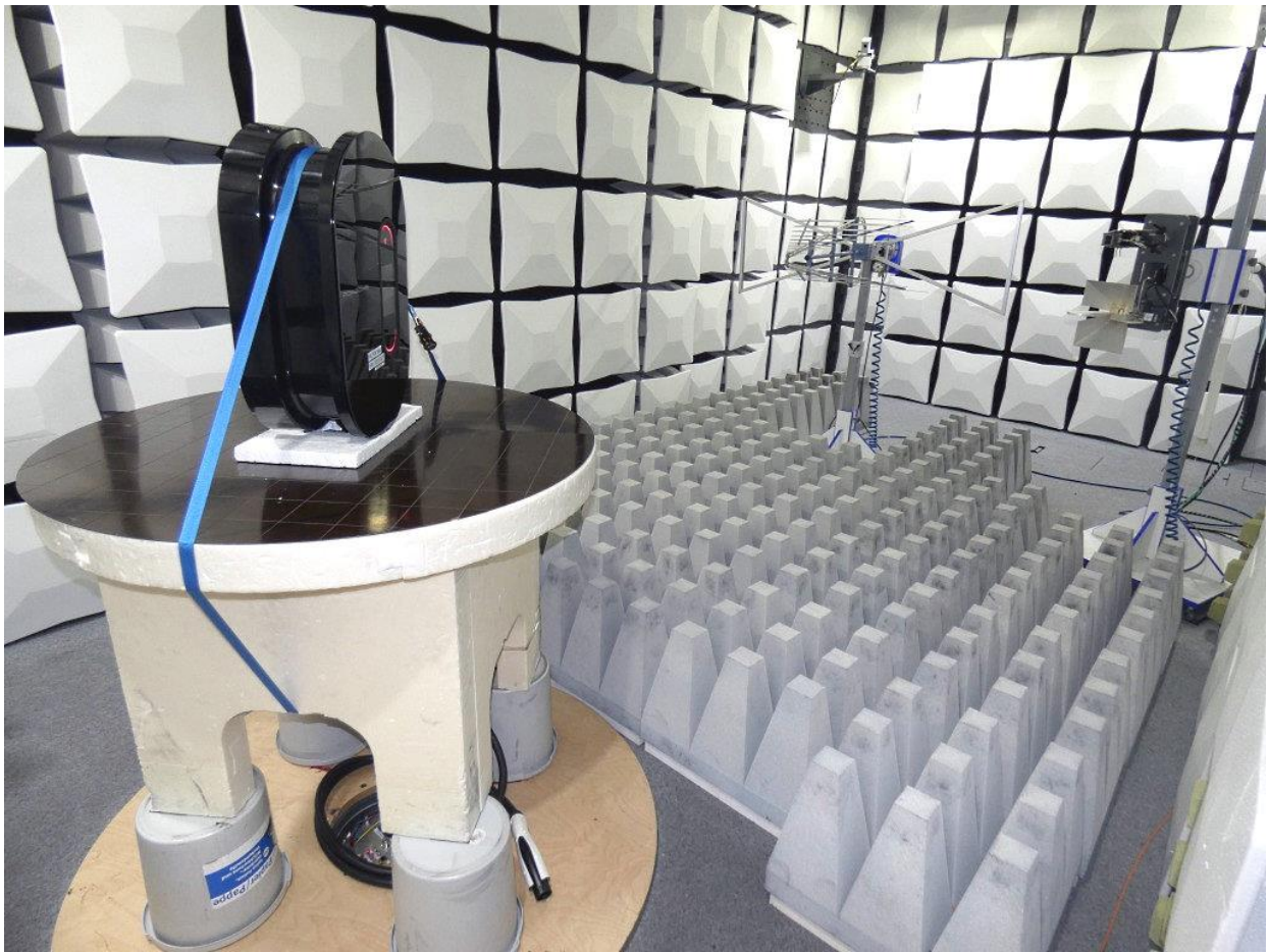
Photo 4: Test setup for radiated measurements in fully anechoic chamber 1 GHz – 26 GHz
