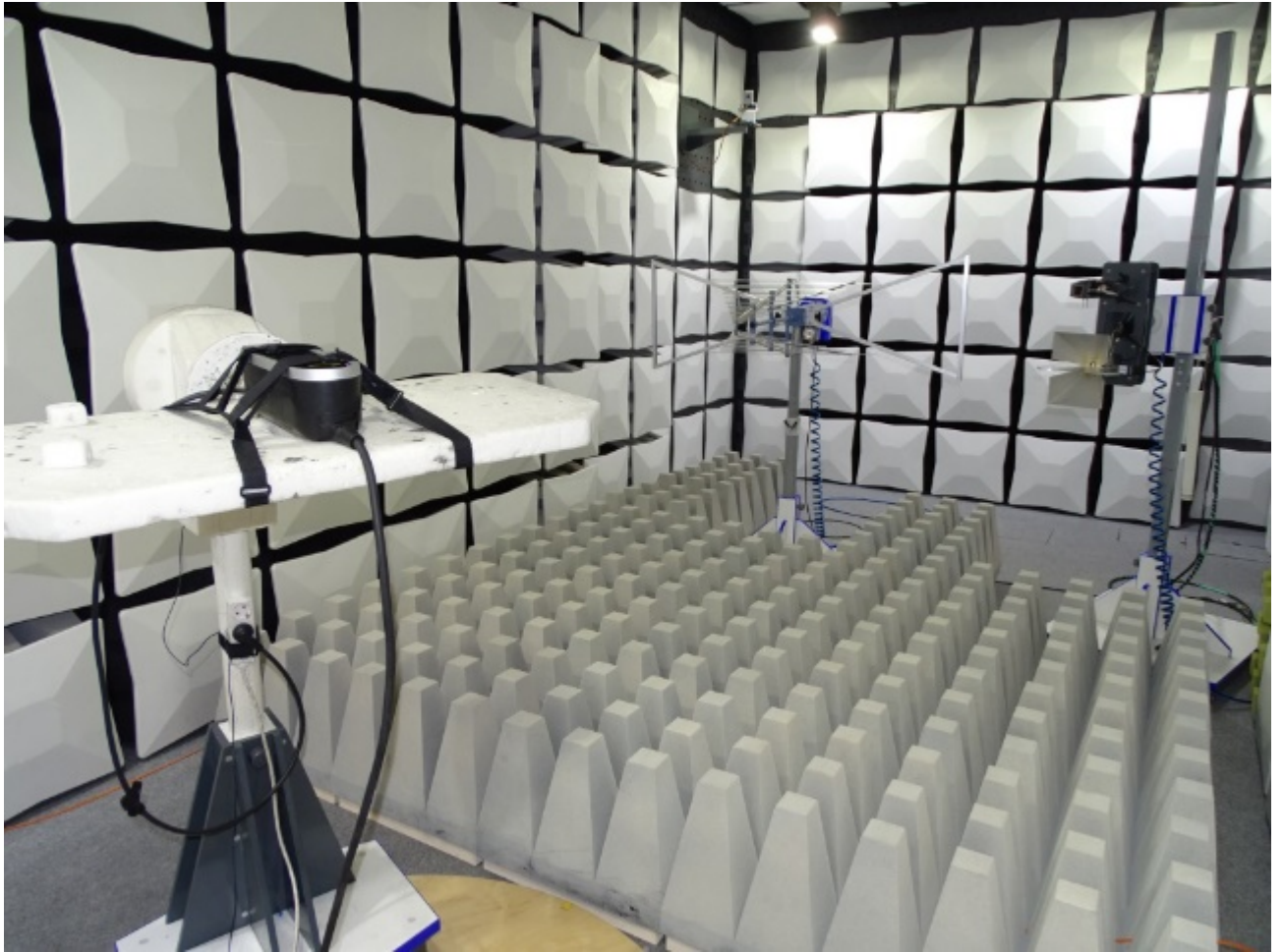
Photo 6: Test setup for radiated measurements in fully anechoic chamber 1 GHz – 26 GHz
