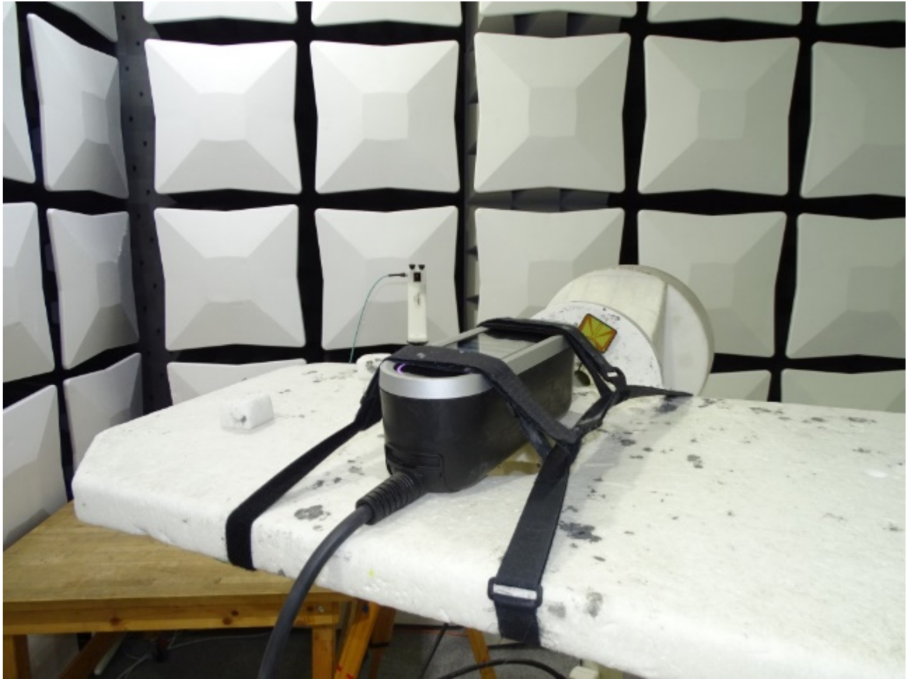
Photo 7: Test setup for radiated measurements in fully anechoic chamber above 26 GHz
