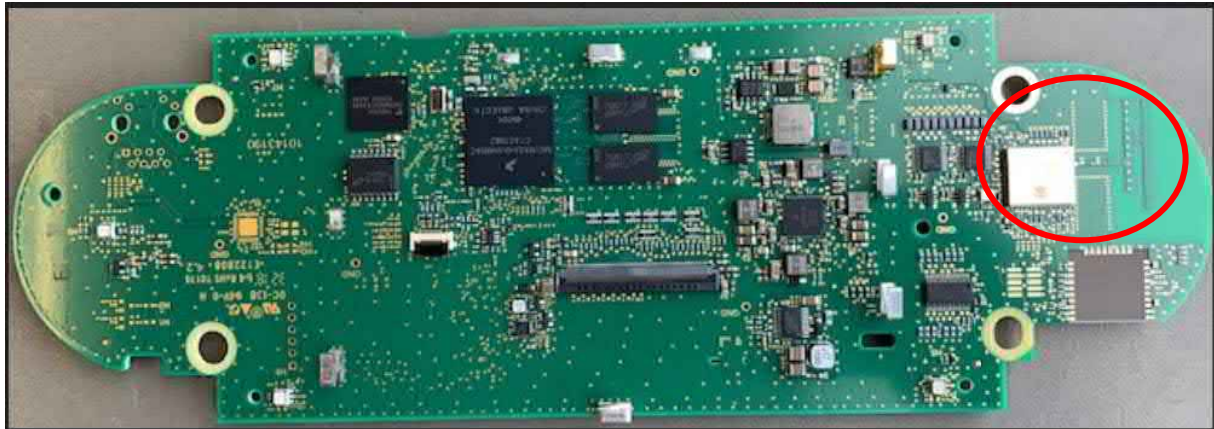
Picture 1: Front View (COM-Board with WLAN-module and antenna → red higlighted)
