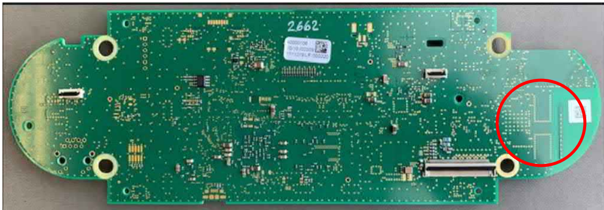
Picture 2: Back View (COM-Board with antenna → red highlighted)
