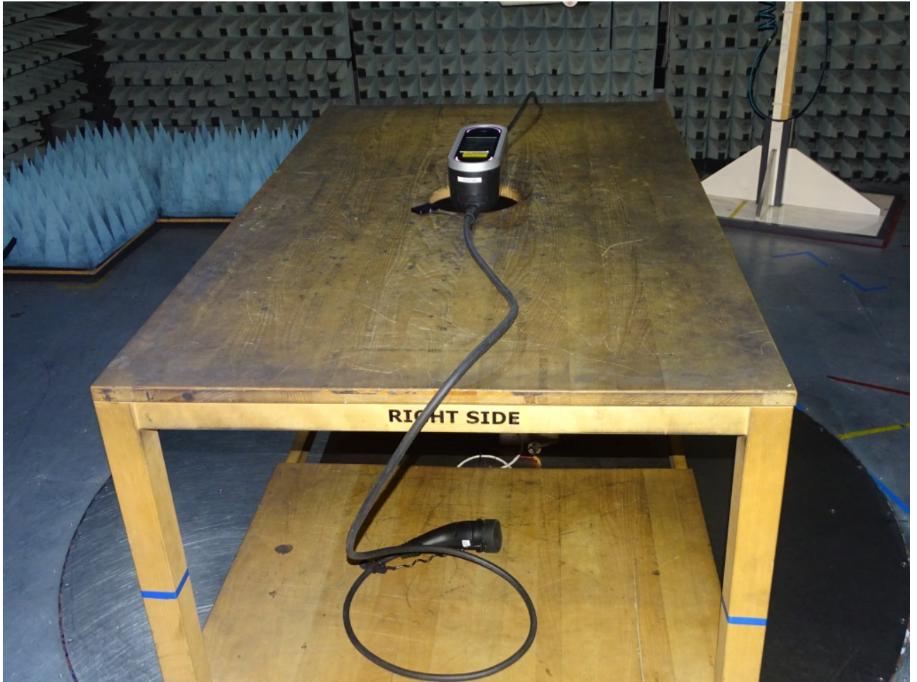
Photo 2: Test setup for radiated measurements in semi anechoic chamber, side view
