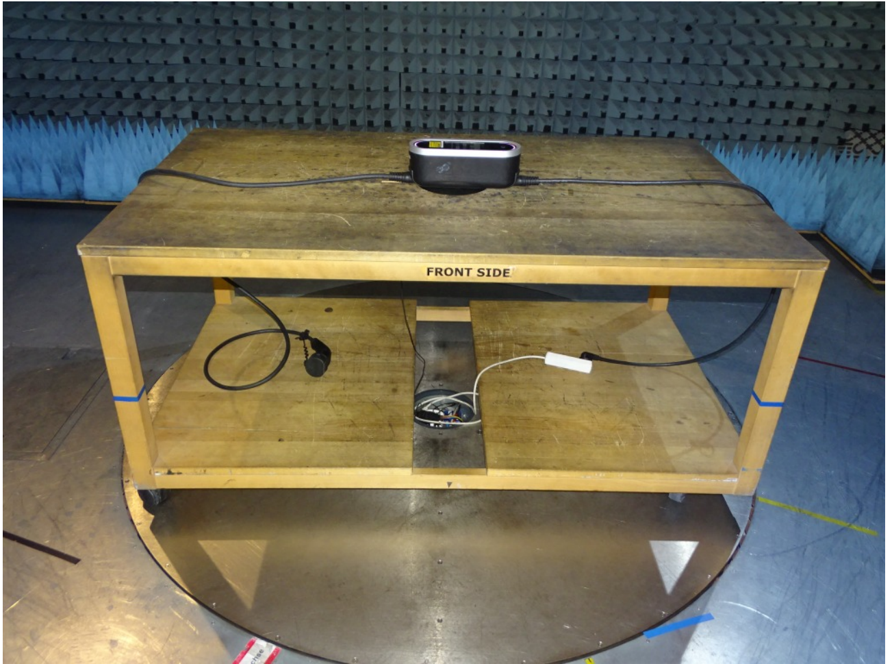
Photo 1: Test setup for radiated measurements in semi anechoic chamber, front side view
