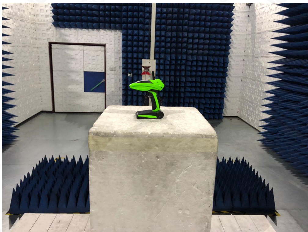
FCC RADIATED EMISSION TEST SETUP ABOVE 1GHZ
