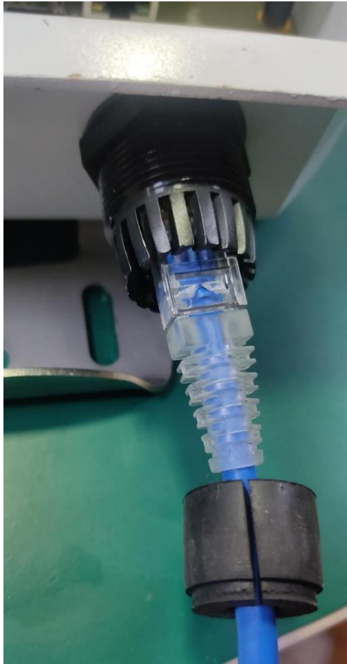
Figure: Procedure for connecting the RJ45 cable (ethernet)
