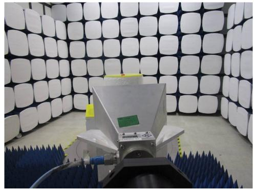
1.3 Radiated Spurious Emissions Test Setup
