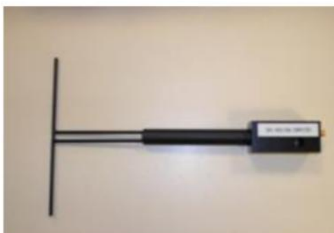
Figure 1 – Satimo COMOSAR Validation Dipole
