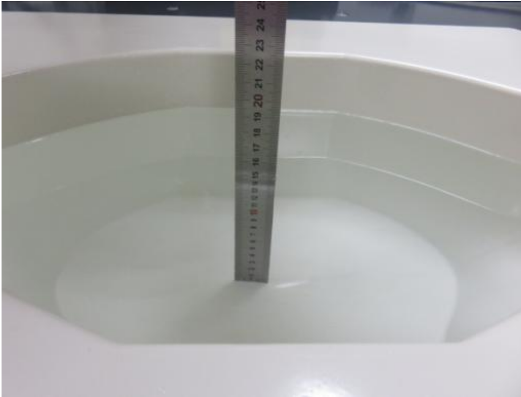
Photograph of the depth in the Body Phantom (2450MHz, 15.5cm depth)
