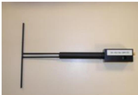
Figure 1 – Satimo COMOSAR Validation Dipole
