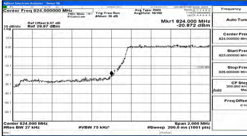
Band Edge Test Graph(s) (Channel Bandwidth: 1.4 MHz)_LCH_QPSK
