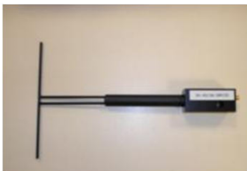
Figure 1 – Satimo COMOSAR Validation Dipole
