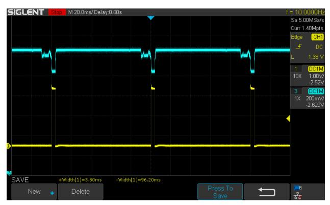
The blue trace represents the Device VCC after a 15 ohm supply series resistor. The yellow trace represents the radio TX active high signal.
