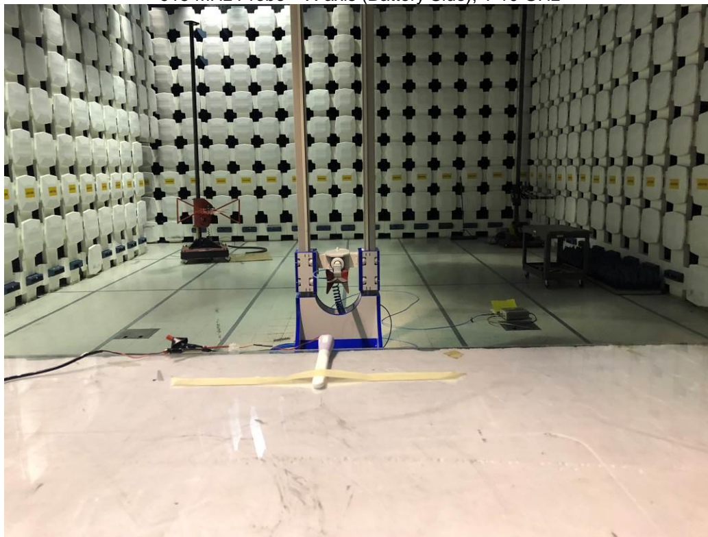
915 MHz Probe – X-axis (Battery Side), 1-10 GHz
