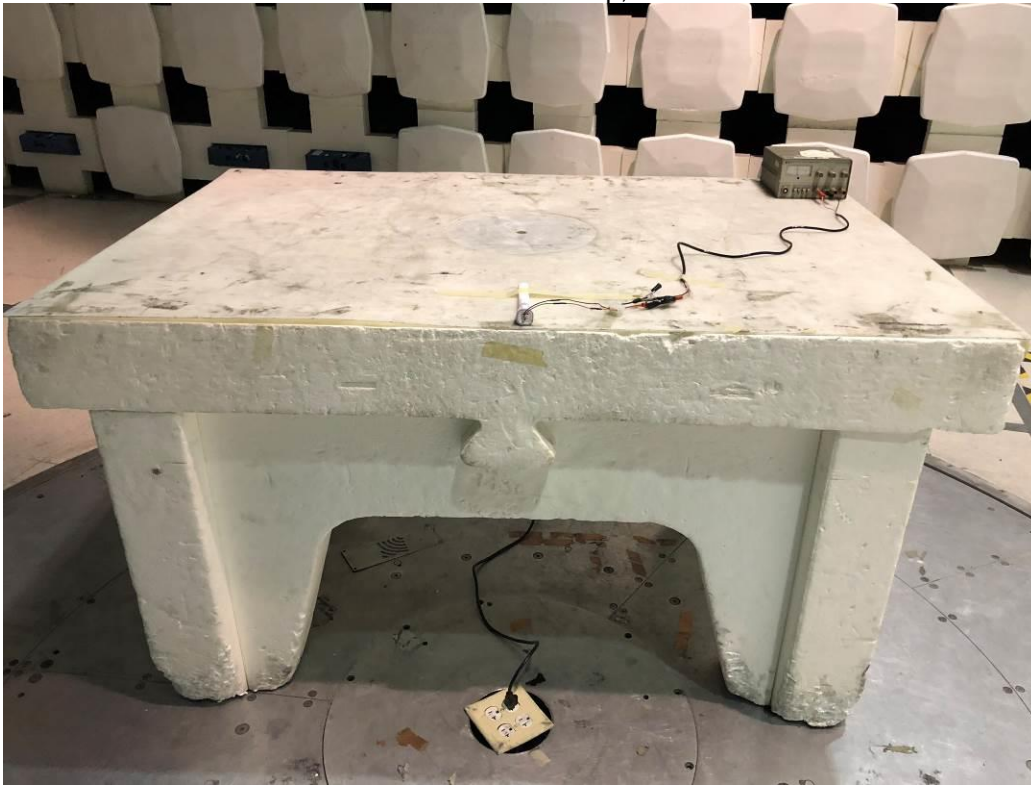
Radiated Emissions Test Setup, 30-1000 MHz
