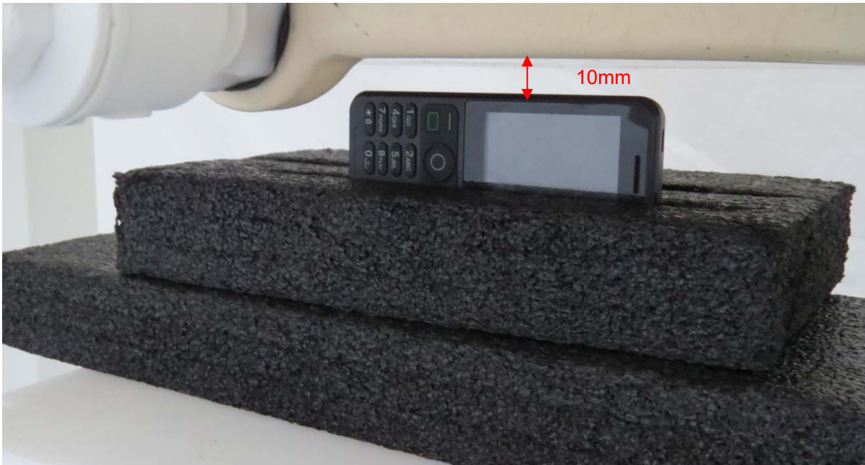
Picture 7: Left Edge, the distance from handset to the bottom of the Phantom is 10mm
