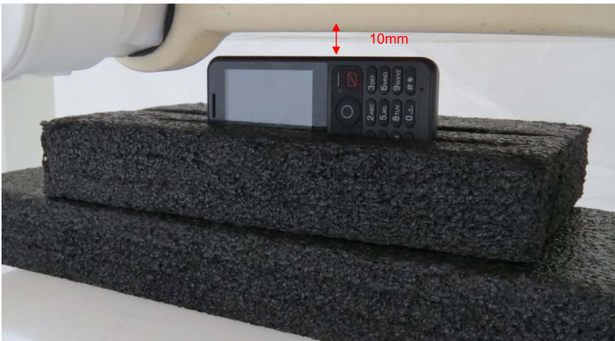
Picture 8: Right Edge, the distance from handset to the bottom of the Phantom is 10mm
