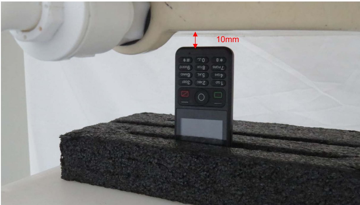
Picture 10: Bottom Edge, the distance from handset to the bottom of the Phantom is 10mm
