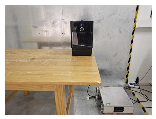
Set-up for Conducted RF test at Antenna Port
