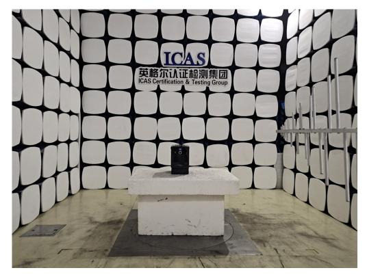
**Set-up for Spurious Emissions above 1GHz**
