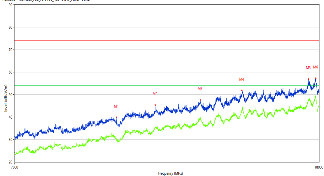
R Emission Test case_FCC_Part 15C_FCC 15.247_7GHz-18GHz
