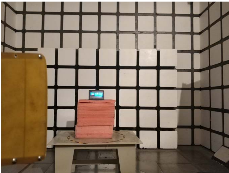
Radiated Emissions View (Above 1 GHz)
