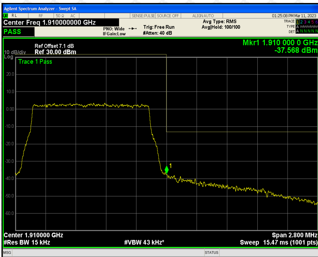
Band2 QPSK BW=3MHz Channel=18615 RB Size=15 Position=#0
