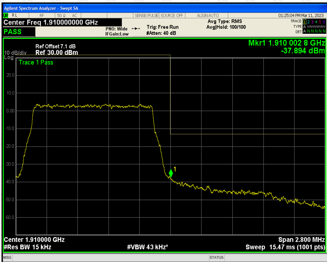
Band2 QAM16 BW=1.4MHz Channel=19193 RB Size=6 Position=#0
