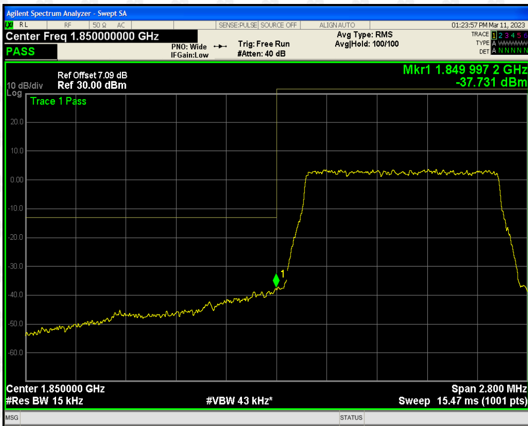
Band2 QAM16 BW=1.4MHz Channel=18607 RB Size=6 Position=#0
