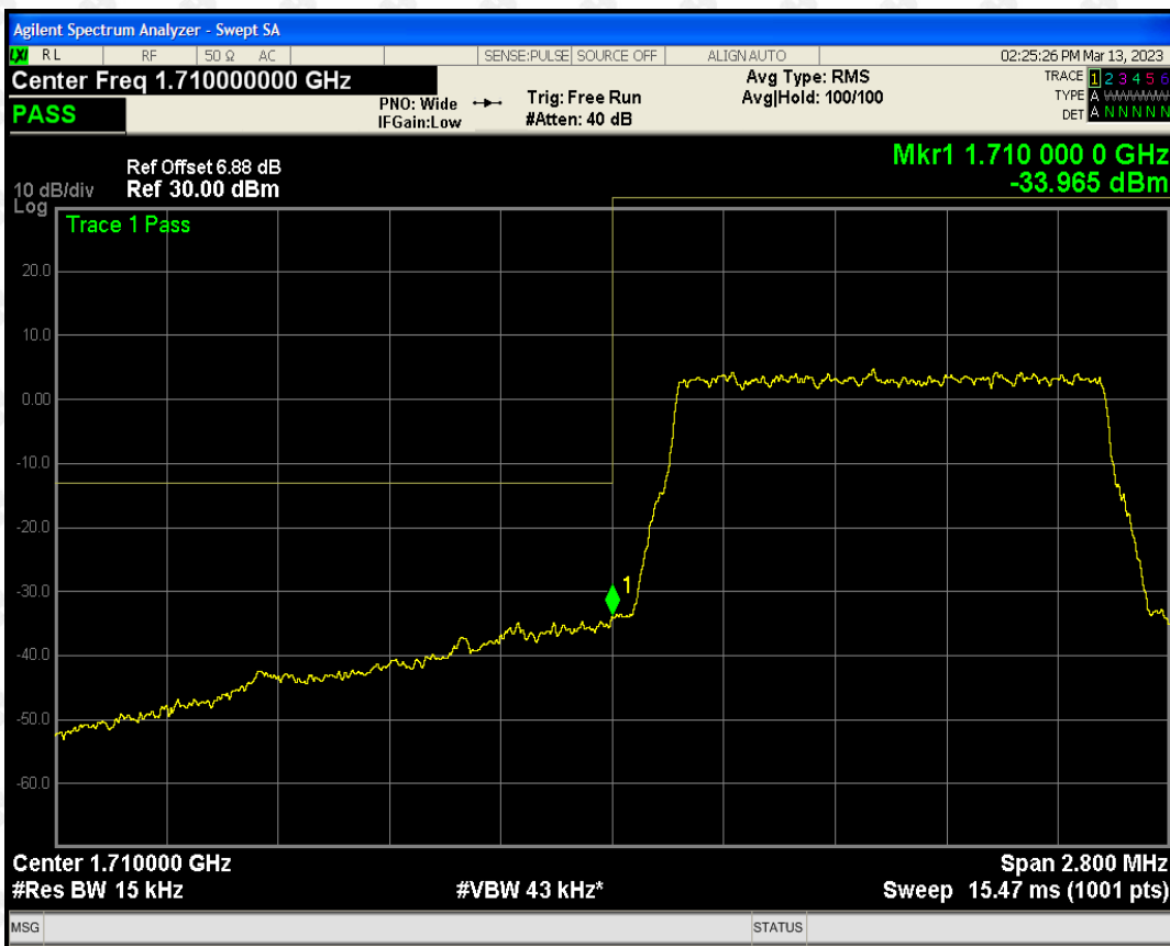
Band66 QPSK BW=1.4MHz Channel=132665 RB Size=6 Position=#0
