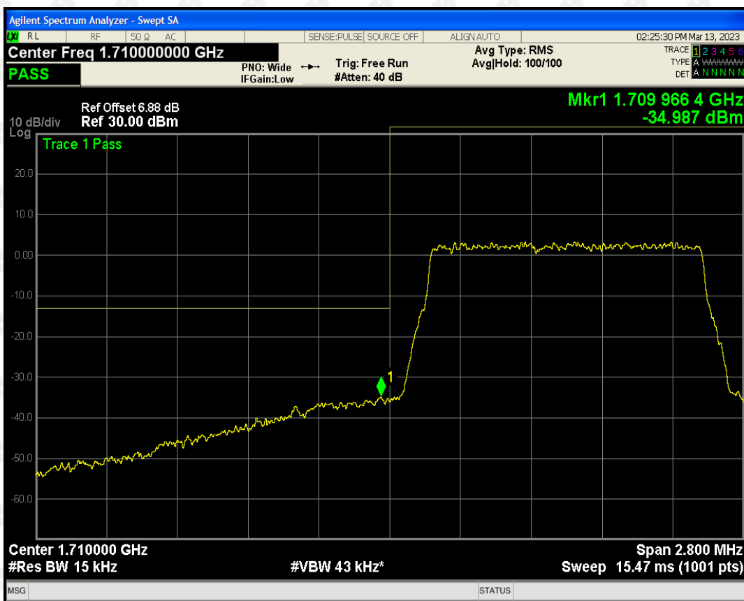
Band66 QAM16 BW=1.4MHz Channel=132665 RB Size=6 Position=#0
