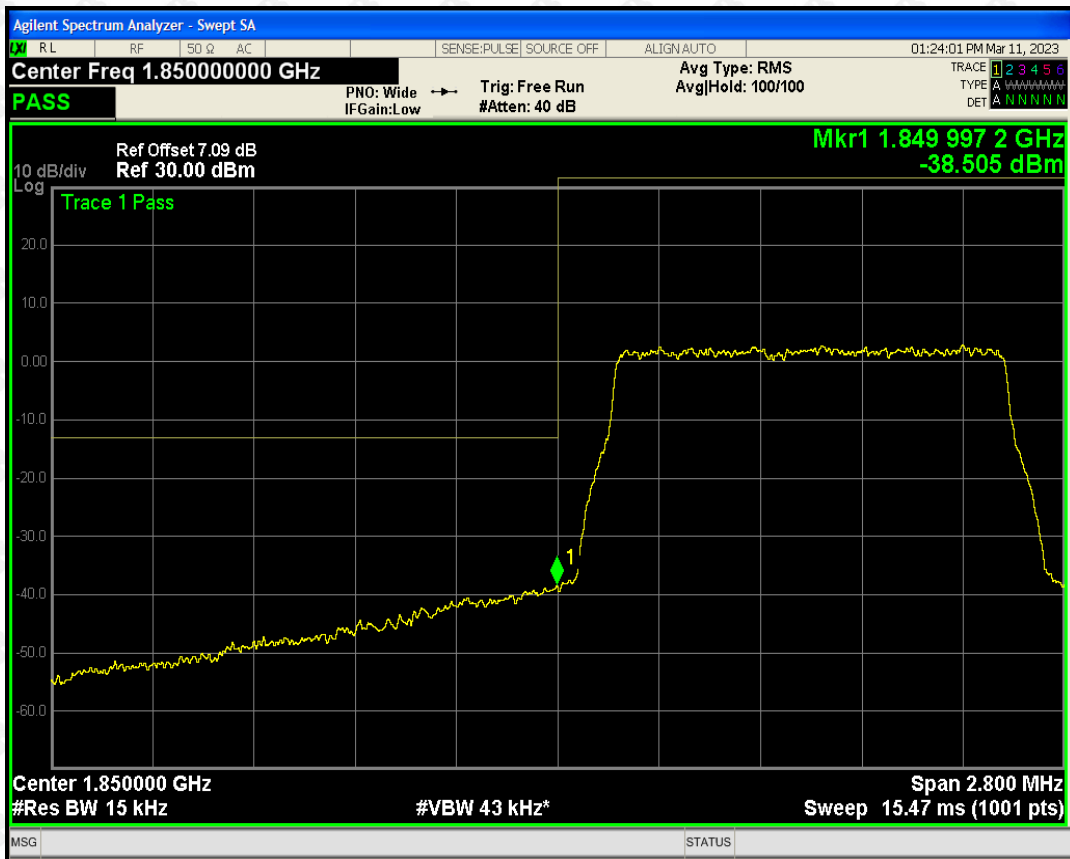
Band2 QPSK BW=1.4MHz Channel=19193 RB Size=6 Position=#0
