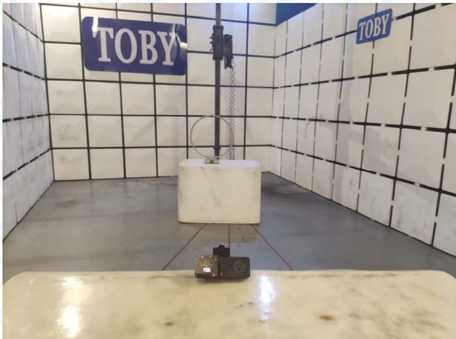
Photo of Setup for Radiated Emission (9KHz-30MHz)
