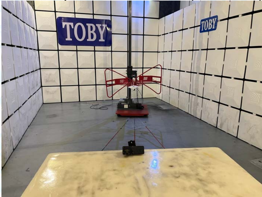
Photo of Setup for Radiated Emission (9KHz-30MHz)
