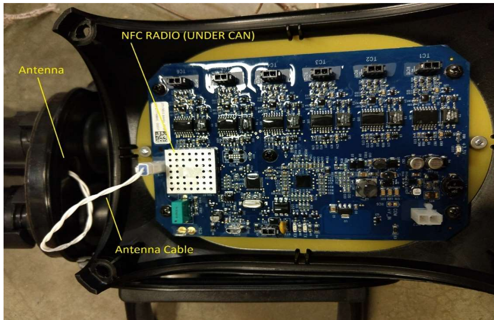
Interior photo of ArcReach Heater Extension Cable (board w/NFC)
