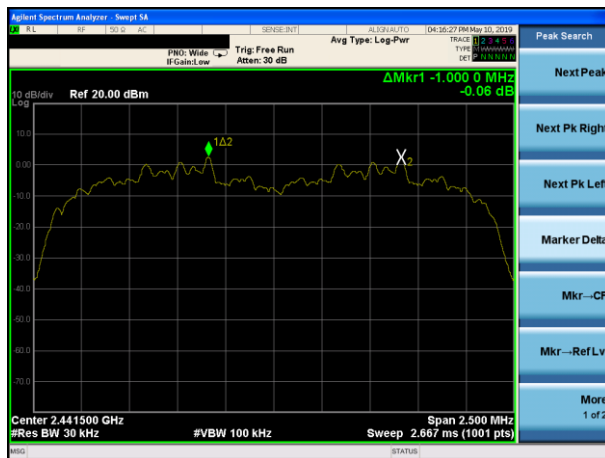
(3Mbps) Channel Separation plot on channel 39-40
