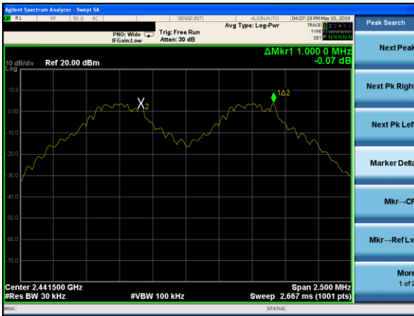
(1Mbps) Channel Separation plot on channel 77-78
