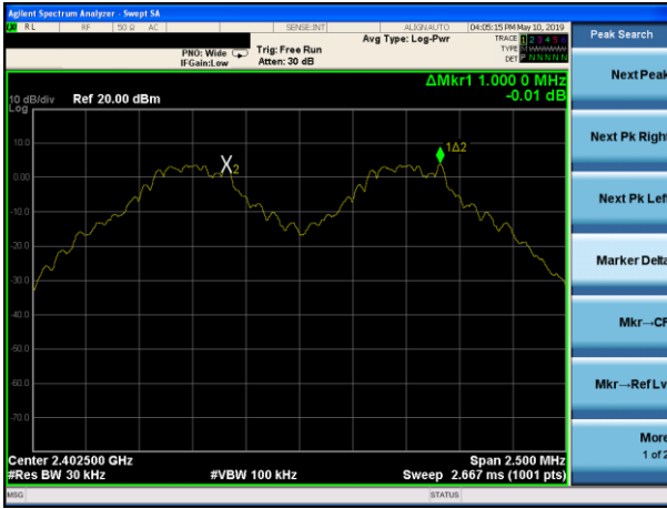
(1Mbps) Channel Separation plot on channel 39-40
