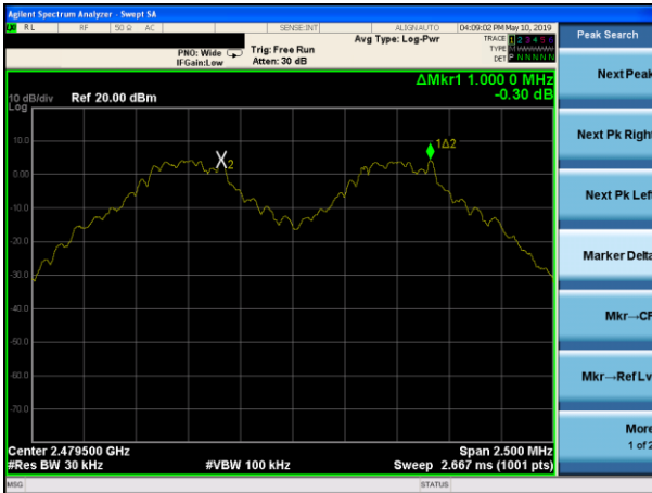
(1Mbps) Channel Separation plot on channel 77-78
