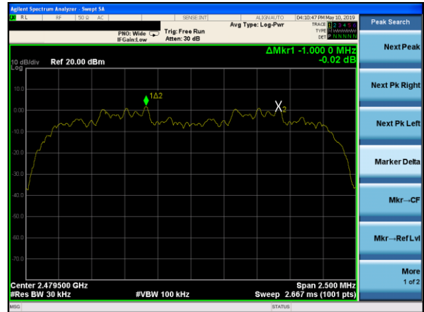
(2Mbps) Channel Separation plot on channel 77-78
