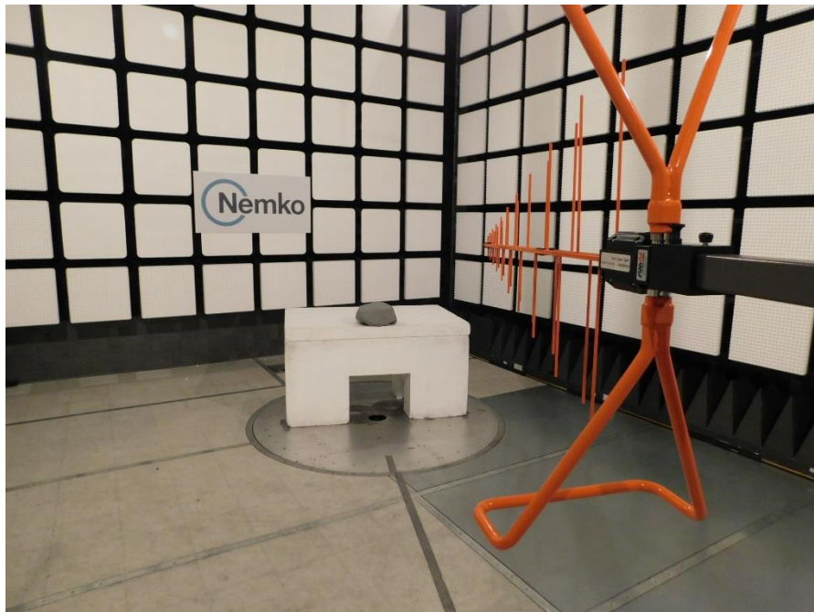
Figure 8.1-3: Radiated emissions setup photo – below 1 GHz
