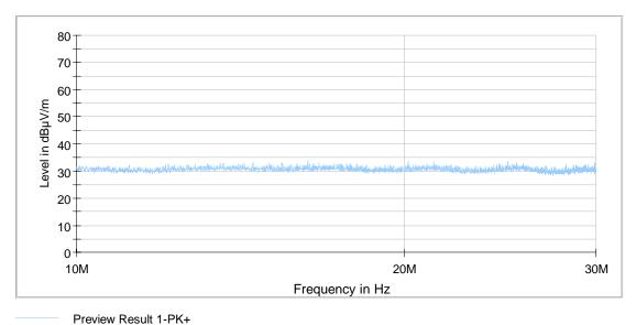
No emissions above the noise floor of the measurement system (max. 33 dB $\mu$ V/m (measured with peak detector at 3 m distance)) found during the preliminary measurement. So no final measurements on the outdoor test site were carried out.
