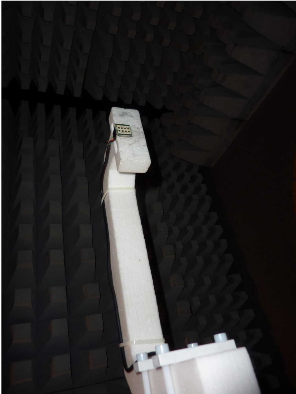
181710_r.jpg: K-LD2, test setup fully anechoic chamber
