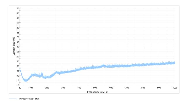
No emissions above the noise floor of the measurement system (max. 25 dB $\mu$ V/m (measured with peak detector at 3 m distance)) found during the preliminary measurement. So no final measurements on the open area test site were carried out.
