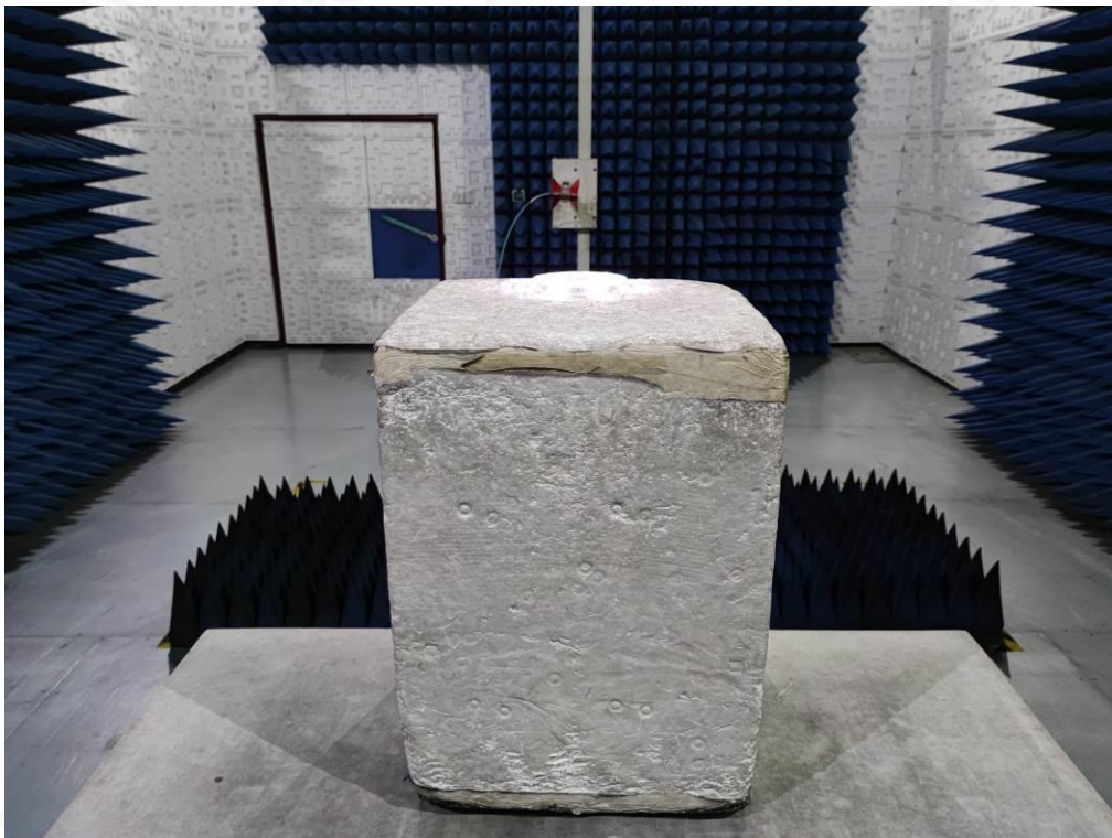
RADIATED EMISSION TEST SETUP ABOVE 1GHZ
