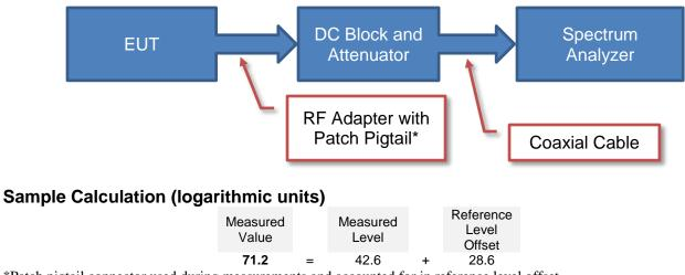
\*Patch pigtail connector used during measurements and accounted for in reference level offset.
