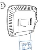
Slide the T-rail mount into the slot of the Access Point.
