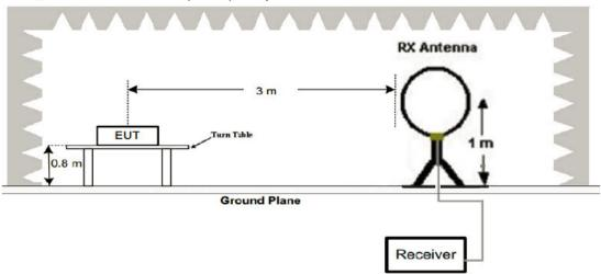
2. Radiated Emission Test-Up Frequency 30MHz~1GHz
