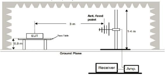
3. Radiated Emission Test-Up Frequency Above 1GHz
