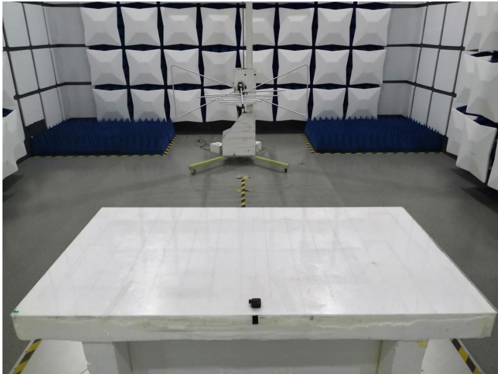
Radiated Emission Below 1GHz
