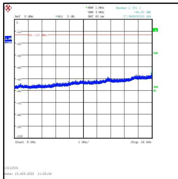
**Transmitter Out of Band Radiated Emissions (GSM 850 & Bluetooth LE) continued**
