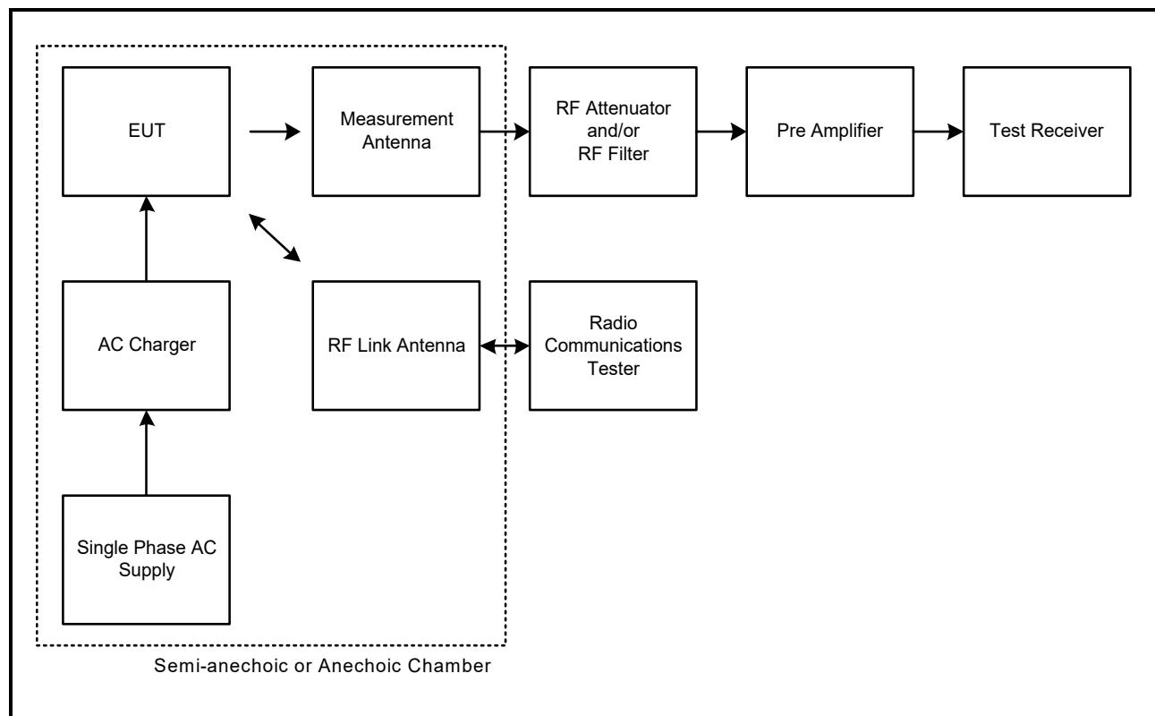
**Test Setup for Transmitter Radiated Emissions (Continued)****Measurements 8 GHz – 18 GHz**
