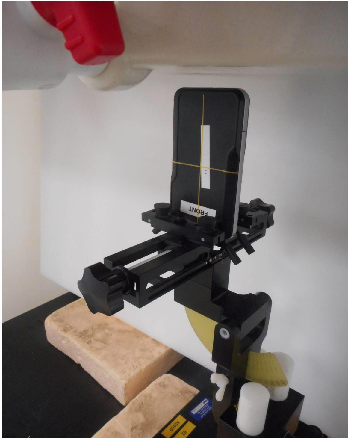
PHT/006: Edge 4 (Left) of DUT Facing Phantom at 10mm
