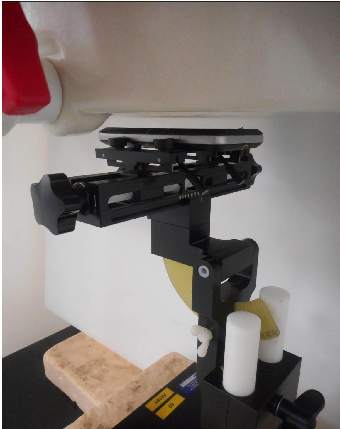
PHT/003: Back of DUT Facing Phantom at 10mm
