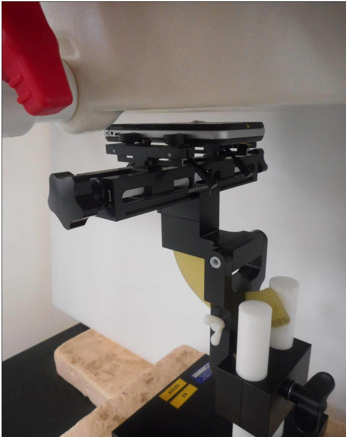
PHT/004: Edge 2 (Right) of DUT Facing Phantom at 10mm
