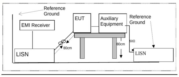
The spectrum was scanned from 150 kHz to 30 MHz with 200 msec sweep time. The frequency producing the maximum level was re-examined using the EMI test receiver. (Rohde & Schwarz ESR3 and ESR7). The detector functions were set to CISPR quasi-peak
