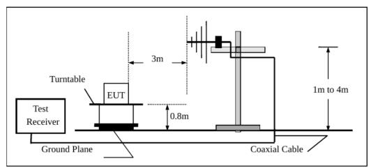
At frequencies below 1000 MHz, measurements performed using the CISPR quasi-peak detection. At frequencies above 1000 MHz, measurements performed using the peak and average measurement procedures described in KDB "558074 D01 15.247 Meas Guidance v05"
