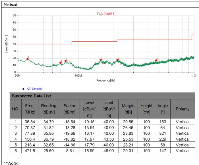
1. Level  $[dB\mu V/m]$  = Reading  $[dB\mu V]$  + Factor [dB/m]
