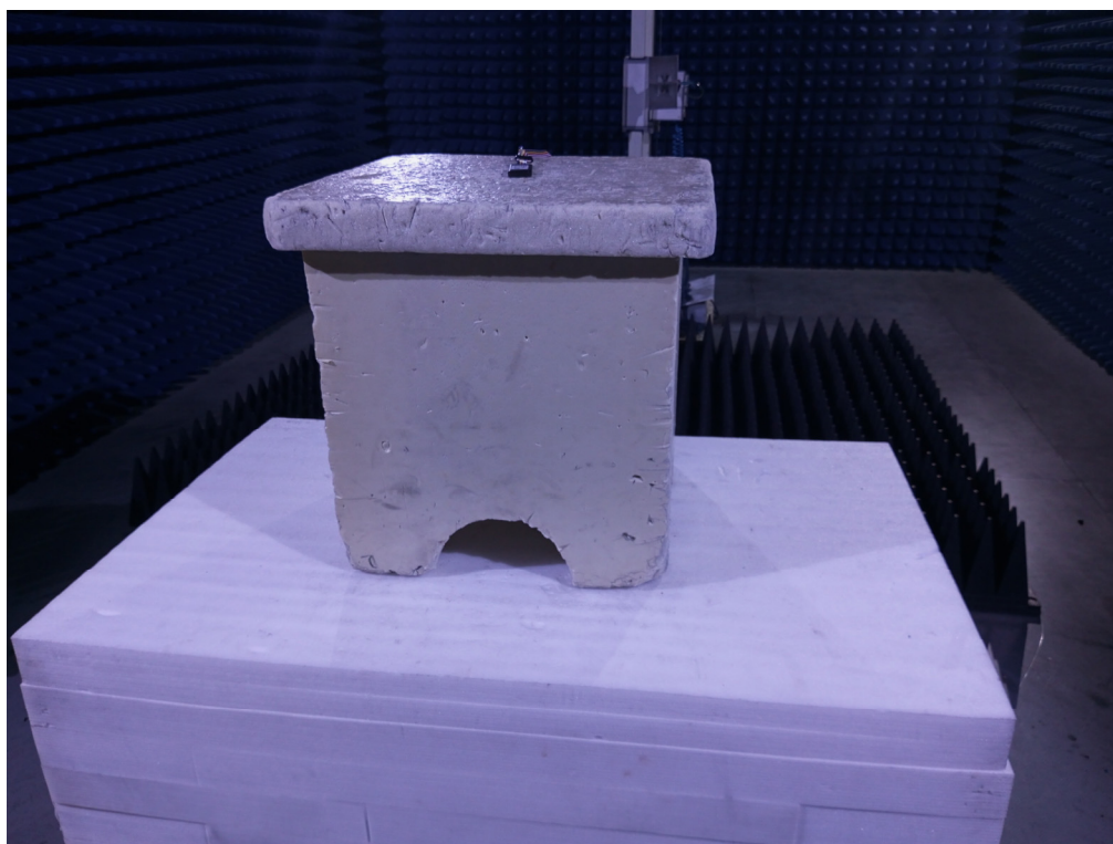
Photo of Radiated Emission Measurement (Above 1G)
