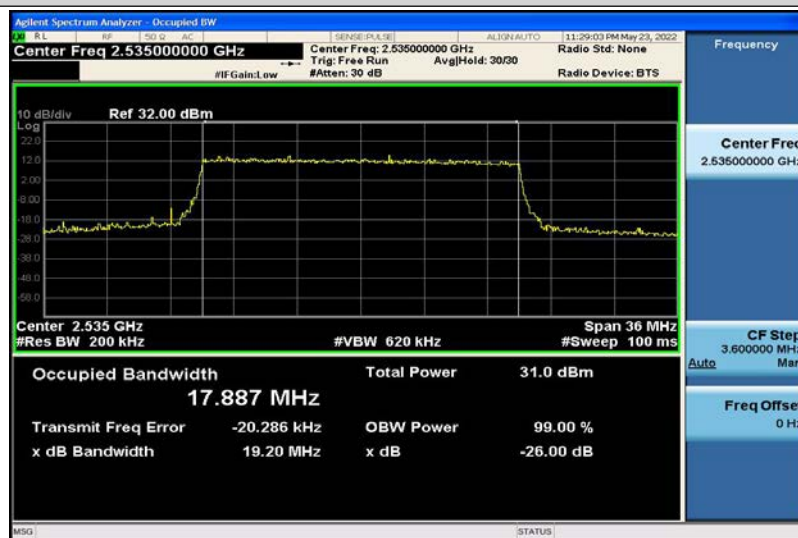
Band7-20MHz-QPSK-21100-100RB#0-17.887
