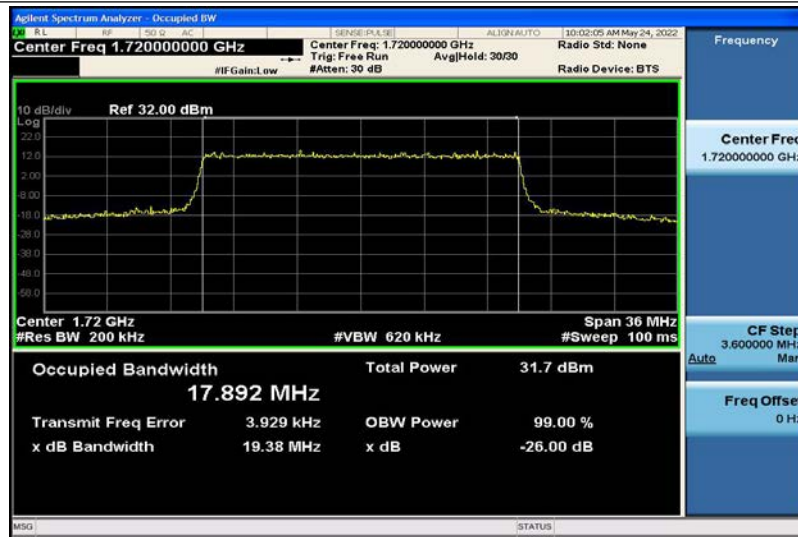
Band4-20MHz-QPSK-20050-100RB#0-17.892
