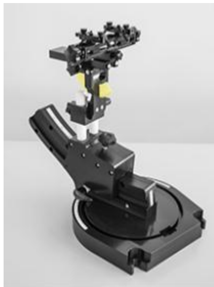
Device holder supplied by SPEAG
