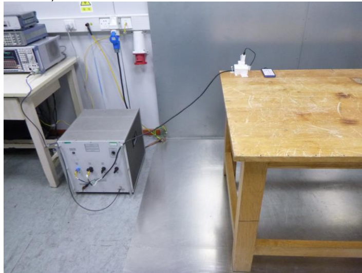
Radiated Emissions (30MHz-1GHz)
