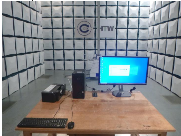
Radiated Emissions (30MHz-1GHz)
