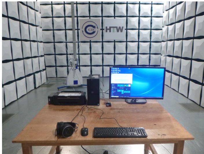
Radiated Emissions (30MHz-1GHz)
