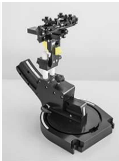
Device holder supplied by SPEAG
