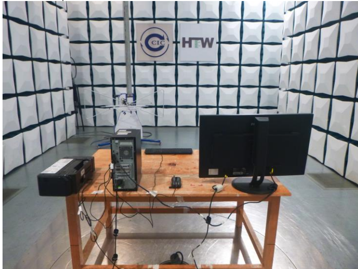
Radiated Emissions (30MHz-1GHz)
