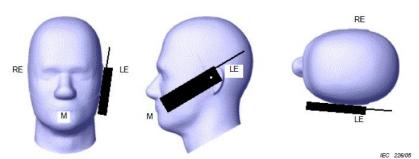
Picture 2 Cheek position of the wireless device on the left side of SAM
