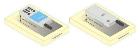
Picture 4 Test positions for body-worn devices
