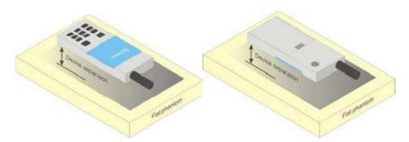
Picture 4 Test positions for body-worn devices
