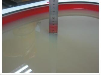
Liquid depth in the Head phantom
