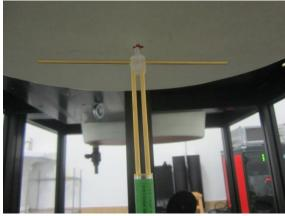
Photo of Dipole Setup
