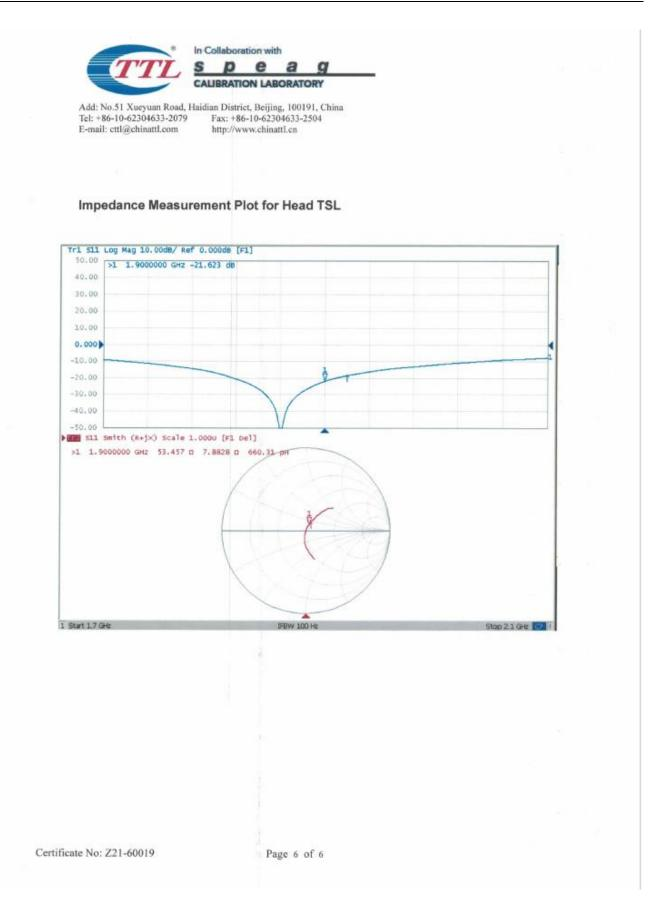
Referring to KDB865664 D01, if dipoles are verified in return loss (<-20dB, within 20% of prior calibration), and in impedance (within 5 ohm of prior calibration), the annual calibration is not necessary and the calibration interval can be extended.
