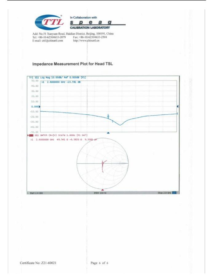
Referring to KDB865664 D01, if dipoles are verified in return loss (<-20dB, within 20% of prior calibration), and in impedance (within 5 ohm of prior calibration), the annual calibration is not necessary and the calibration interval can be extended.
