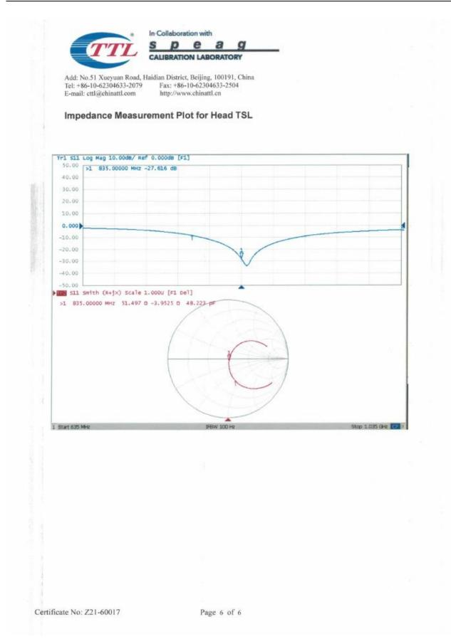
Referring to KDB865664 D01, if dipoles are verified in return loss (<-20dB, within 20% of prior calibration), and in impedance (within 5 ohm of prior calibration), the annual calibration is not necessary and the calibration interval can be extended.
