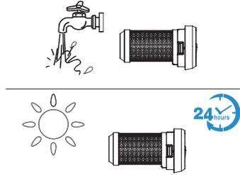
The HEPA filter can be washed under running water and must be completely dry before reinstalling.
