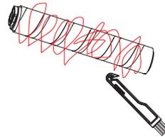
Remove the debris wrapped around the roller with the Tineco Hair Cleaning Tool.
