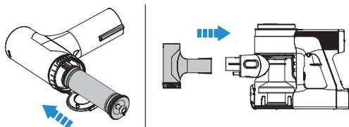
Replace a clean filter to the main body. Put the dirty pre-filter into the cleaning tool and connect the cleaning tool to the main body.
