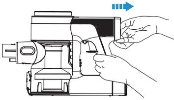
Press the HEPA release button and gently remove for cleaning. Do not use the appliance without first installing the HEPA filter.
