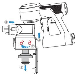
After cleaning, insert the clean pre-filter into mesh filter properly and it clicks into place. Install the clean filters and dustbin back into the main body, then close the dustbin flap.
