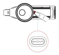
The appliance will start in AUTO mode by default. After 3 seconds, press the MAX/AUTO button to switch to Max mode.
