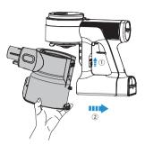
When re-attaching the dustbin, hold on an angle and slot the top of the dustbin into the hook on the main body. Push upwards until the hook is fixed into the slot on the dustbin and then it clicks into place.
