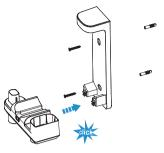
Assemble the two bracket components, with a "click" to signify correct assembly. Once this is complete, use the screws provided by Tineco to affix the dock to the wall.
