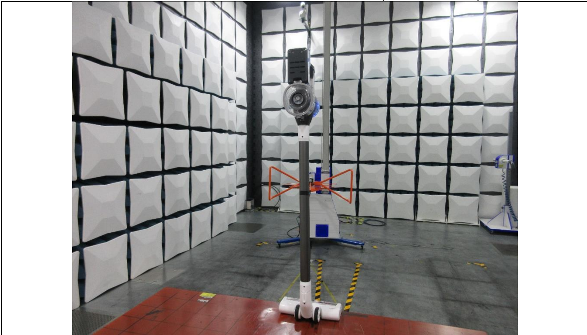
RADIATED RF MEASUREMENT SETUP (30MHz~1GHz)
