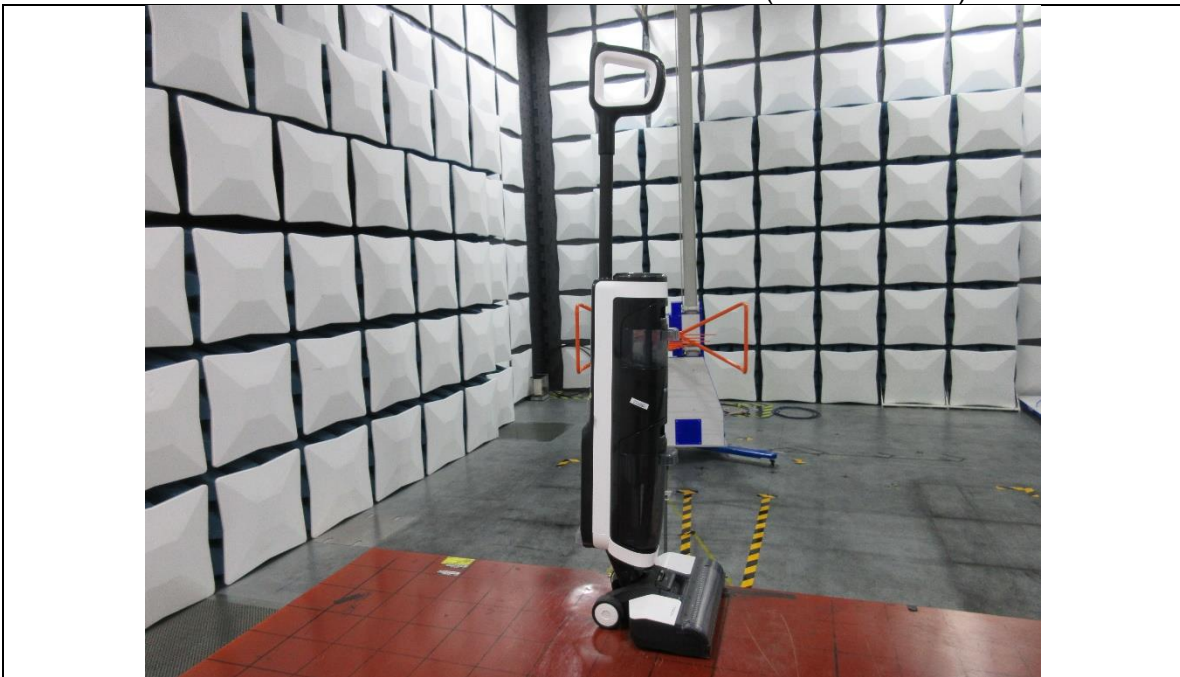
RADIATED RF MEASUREMENT SETUP (30MHz~1GHz)
