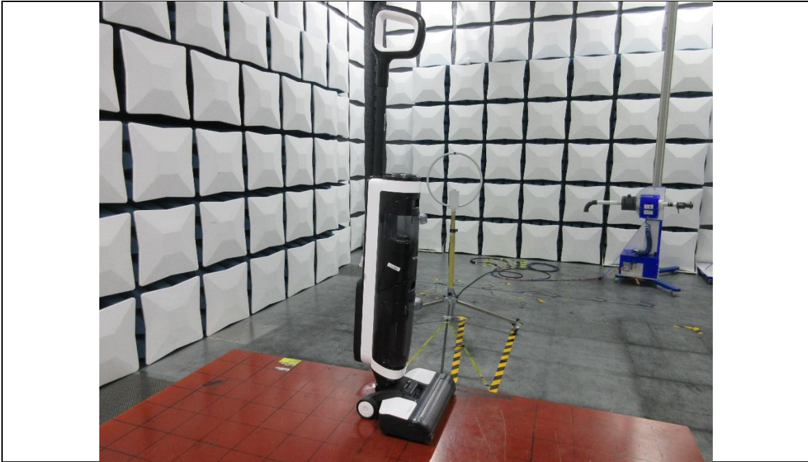
RADIATED RF MEASUREMENT SETUP (Below 30MHz)
