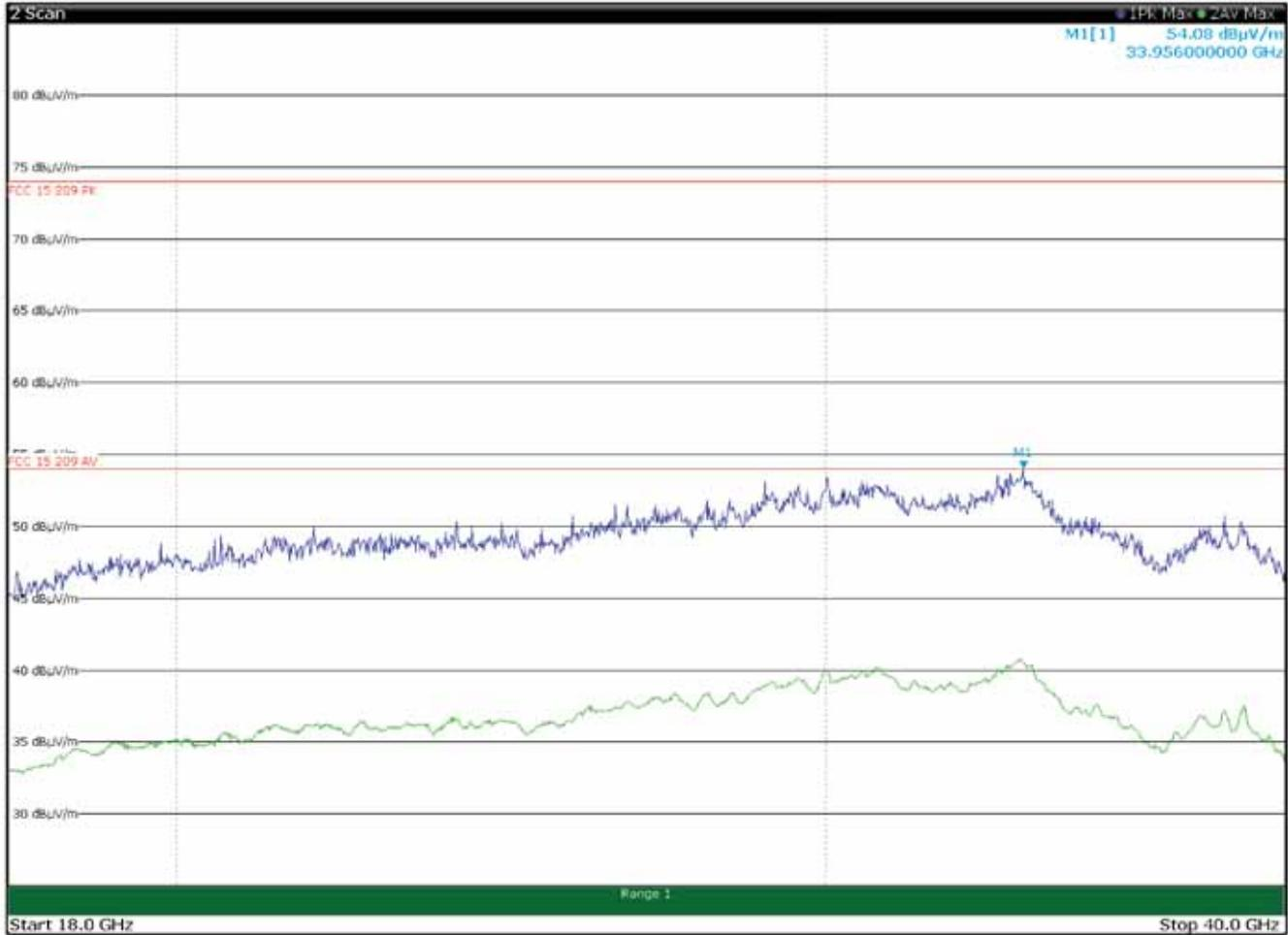
Radiated spurious emissions with antenna in horizontal polarization and with
