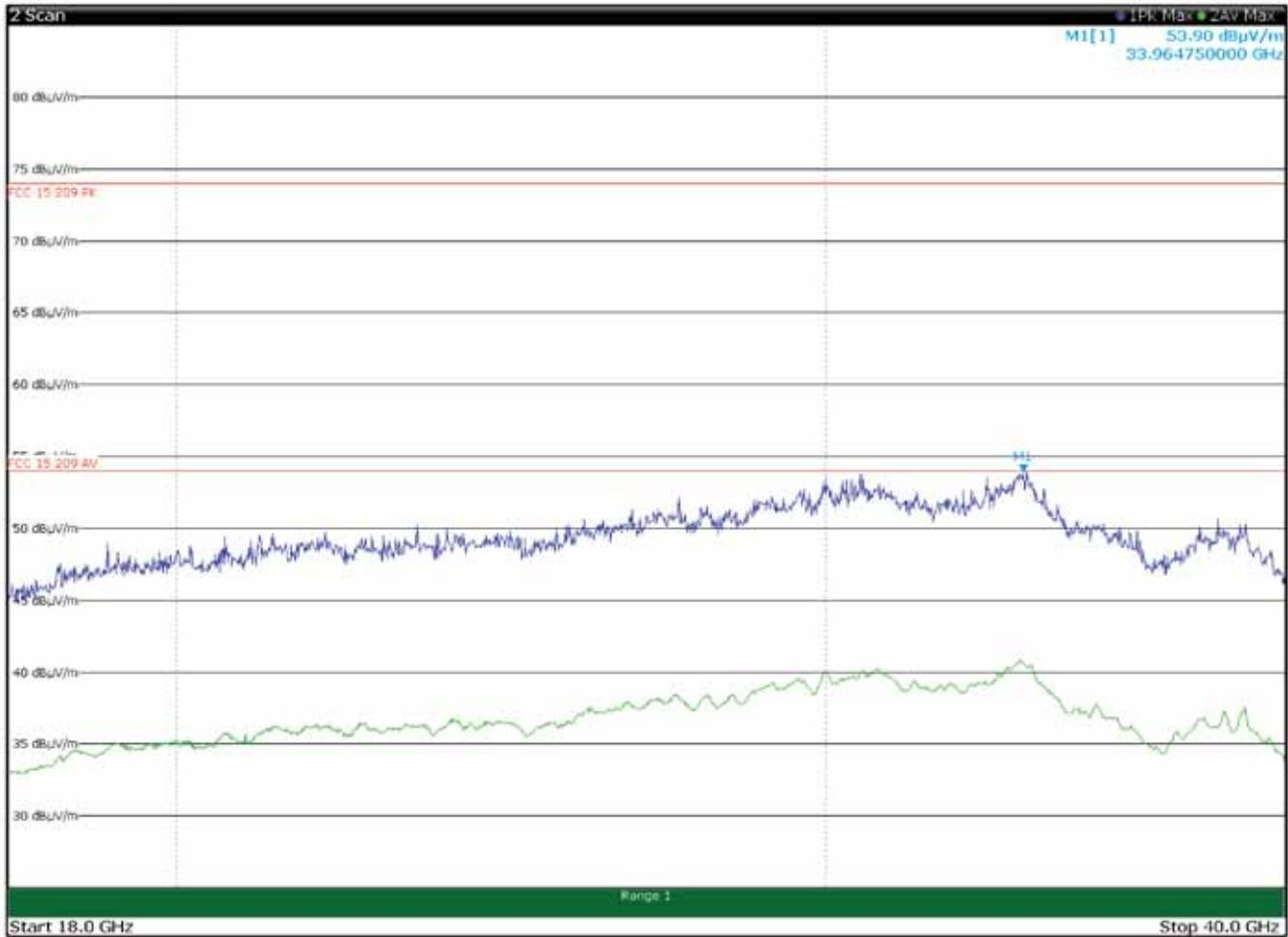
Radiated spurious emissions with antenna in vertical polarization and with
