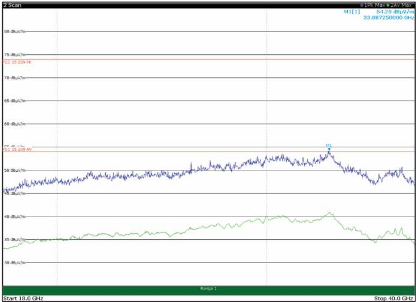
Radiated spurious emissions with antenna in vertical polarization and with WCDMA Tx at 1880 MHz, UHF Tx at 915 MHz, WIFI Tx at 2437 MHz and BT Tx at 2441 MHz (antenna configuration 2)
