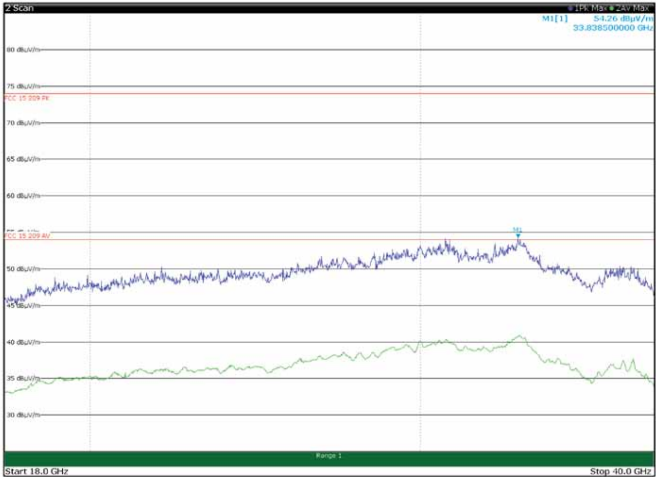
Radiated spurious emissions with antenna in vertical polarization and with WCDMA Tx at 837 MHz, UHF Tx at 915 MHz, WIFI Tx at 5220 MHz and BT Tx at 2441 MHz (antenna configuration 1)
